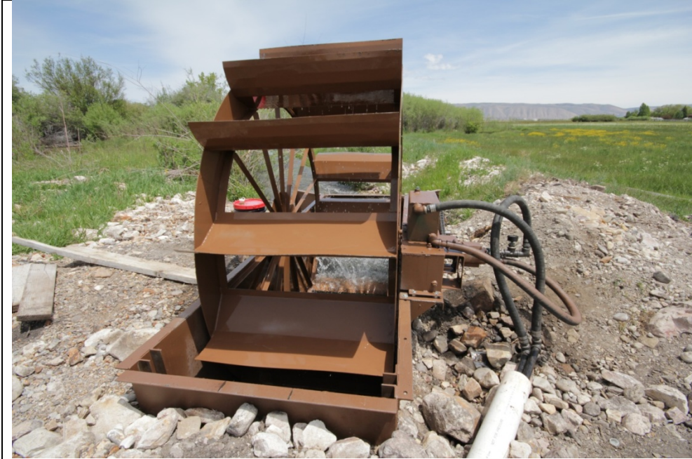
Photo 4: A close-up showing the paddlewheel and hydraulic system.
